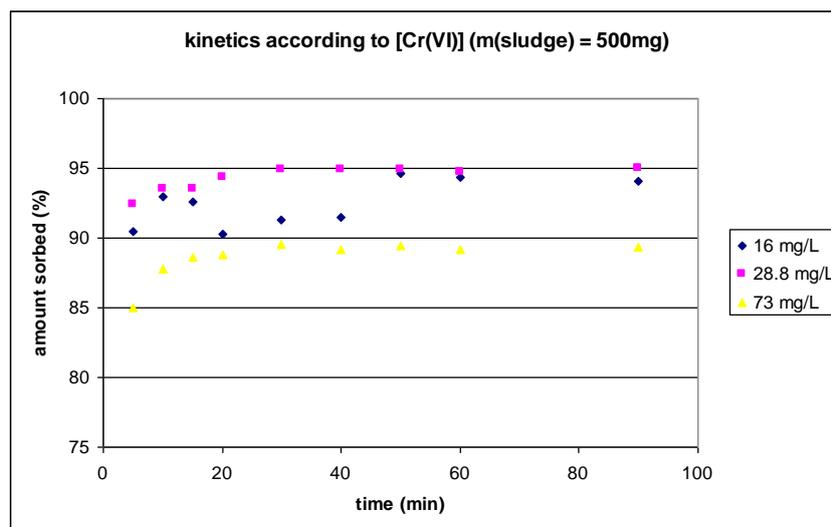
Figure 3 : kinetics according to [Cr<sup>VI</sup>] to a sludge mass 500mg
