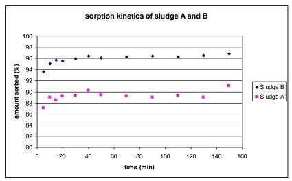
Figure 1: Sorption kinetics of sludge A and B
