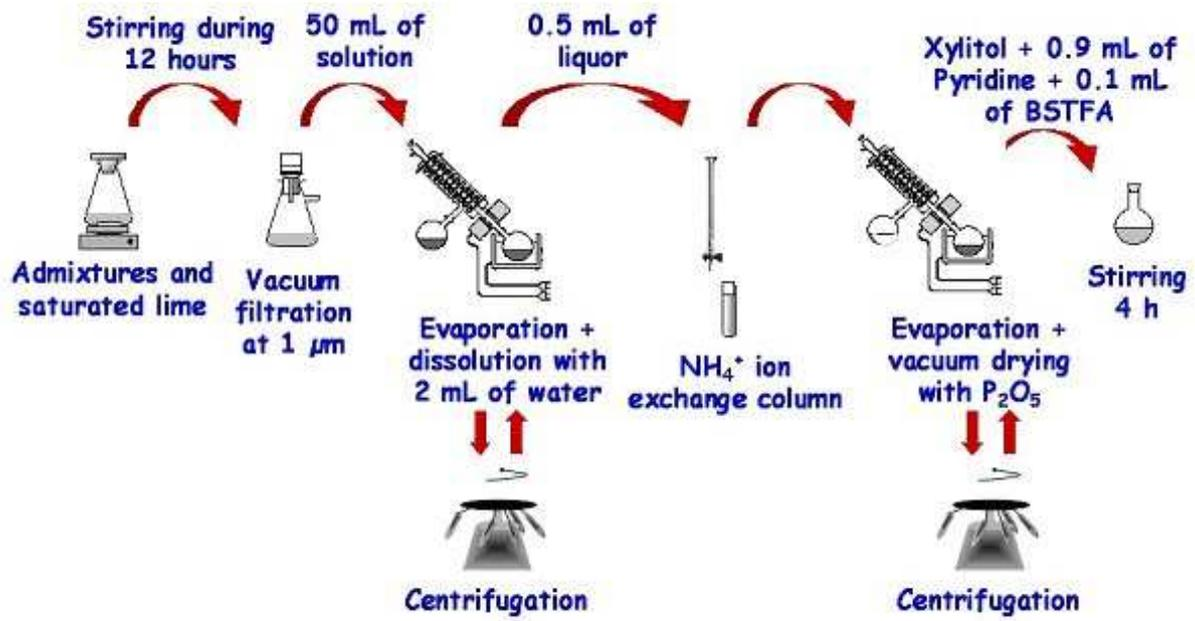
Figure 1 Samples preparation for the analysis of the degradation products.
