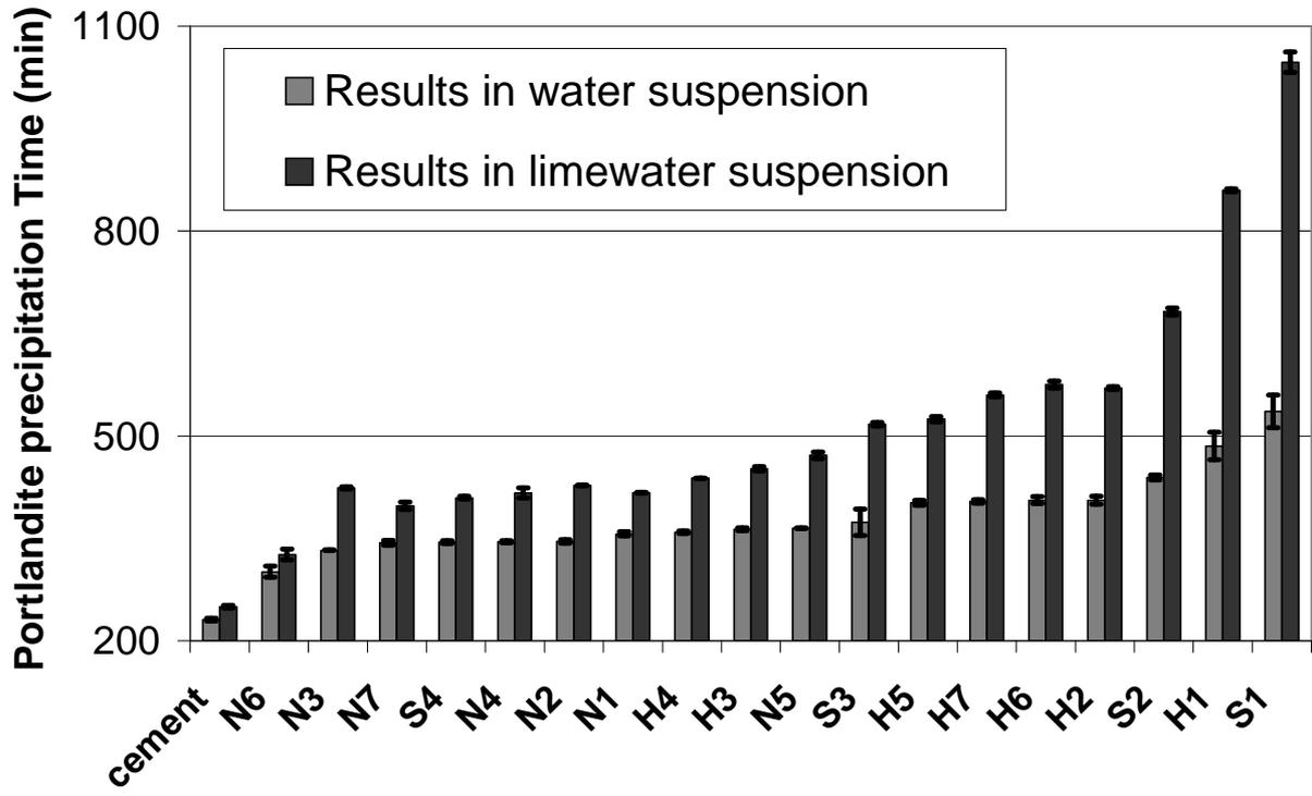
Figure 2. Portlandite precipitation delay in aqueous and limewater system (L/S=20).
