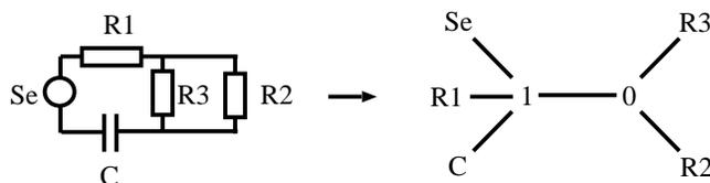
Figure 2: A circuit and an associated bond graph.
