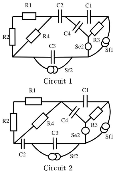
Figure 1: Circuits 1 and 2 are equivalent.
