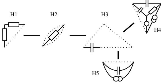
Figure 4: The Tutte decomposition of the circuit 2 of Figure 1 .
