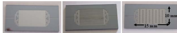
Figure 1: Schematic top view of the "Neutral", "Straight" and "Zigzag" designs, from left to right.
