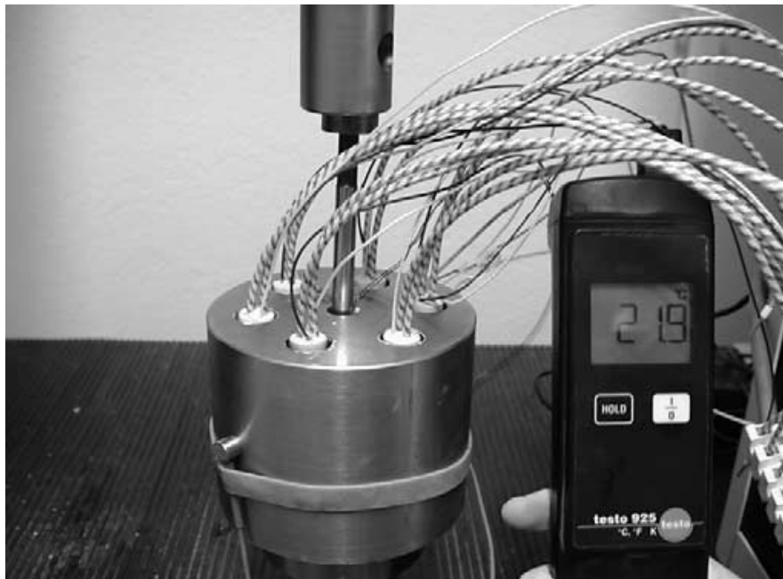
Figure 1: The uniaxial die with the 6 heating rods with a temperature regulation system. The piezoelectric sensor used to detect the acoustic emissions can be seen on the left.
