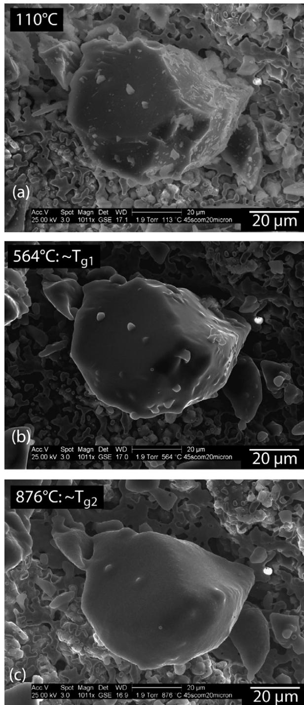
**Figure 2:** ESEM micrographs taken at low magnification on one Bioglass® grain during *in situ* heating from room temperature to 950 °C. Three micrographs have been selected to show the evolution of grain morphology with temperature: 110 °C (a), around  $T_{g1} = 550$  °C (b) and  $T_{g2} = 850$  °C (c).
