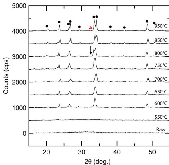
**Figure 4:** Diffractograms of raw and thermally treated bioactive glass 45S5. Under 600 °C the Bioglass® remains amorphous. Over this temperature, crystallization takes place by the formation of  $\text{Na}_2\text{CaSi}_2\text{O}_6$  (•: PDF 77-2189). At 800 °C, the two major peaks of this phase begin to be dissociated while the crystallization of silicorhenanite (▲: PDF 32-1053, isostructural to apatite) begins. At 1050 °C, the material begins the melting process).
