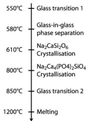
Figure 12: Summary of the structural transformations of 45S5 with temperature.
