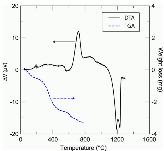
Figure 1: TGA–DTA of 45S5 Bioglass®.
