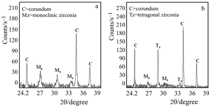
**Fig. 6** X-rays diffraction of the commercial mixture (10 vol% of ZrO<sub>2</sub>) before and after the thermal treatment
