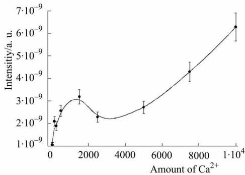
**Fig. 8** Evolution in function of the amount of dopant, of the TL intensity of the peak situated between 70°C and 110°C for  $\alpha$ -Al<sub>2</sub>O<sub>3</sub> doped by Ca<sup>2+</sup>, prepared by a thermal treatment under Ar + 2% H<sub>2</sub>
