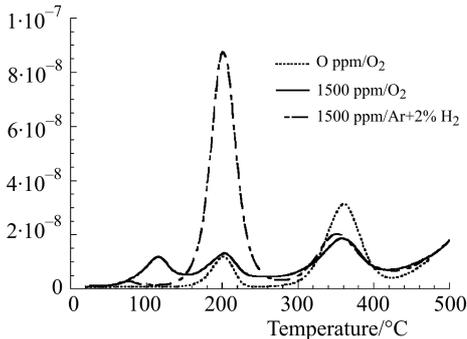
**Fig. 7** TL curves of  $\alpha$ -Al<sub>2</sub>O<sub>3</sub> doped by Ca<sup>2+</sup>, prepared by a thermal treatment under O<sub>2</sub> or Ar + 2% H<sub>2</sub>
