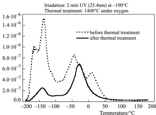
**Fig. 5** Thermoluminescence after UV irradiation of a commercial mixture (allowing the stabilisation of zirconia in tetragonal form after sintering), containing 10 vol% of  $\text{ZrO}_2$ , before and after the thermal treatment
