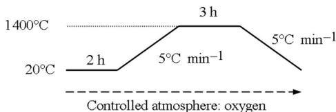
**Fig. 1** Thermal cycle for the treatment of the  $\alpha$ -Al<sub>2</sub>O<sub>3</sub>-ZrO<sub>2</sub> mixtures
