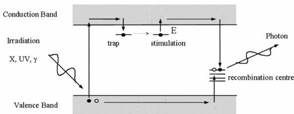
**Fig. 2** Schematic diagram of thermoluminescence mechanism
