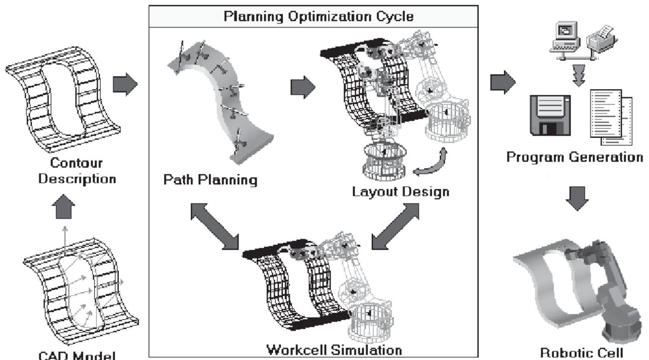
Figure 12. Robotic cell design and programming using Robomax/Laser.
