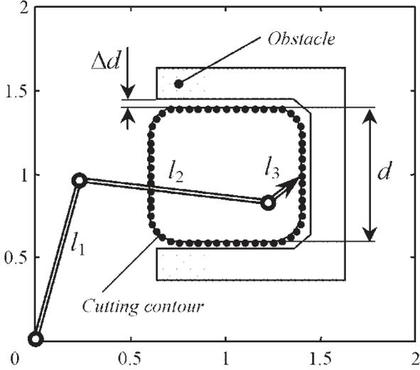
Figure 5. A planar three degree of freedom illustrative example.
