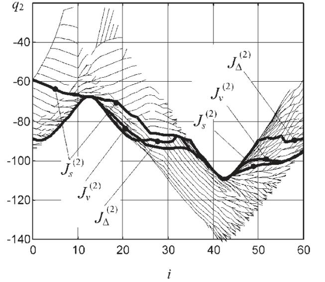
Figure 7. Optimal solutions for the coordinate  $q_2$ .
