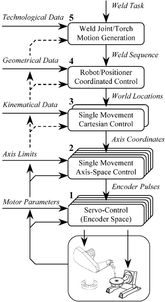
Fig. 2. Multi-level control hierarchy.
