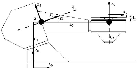
Fig. 7. The coordinate frames of the 2-axis positioner.
