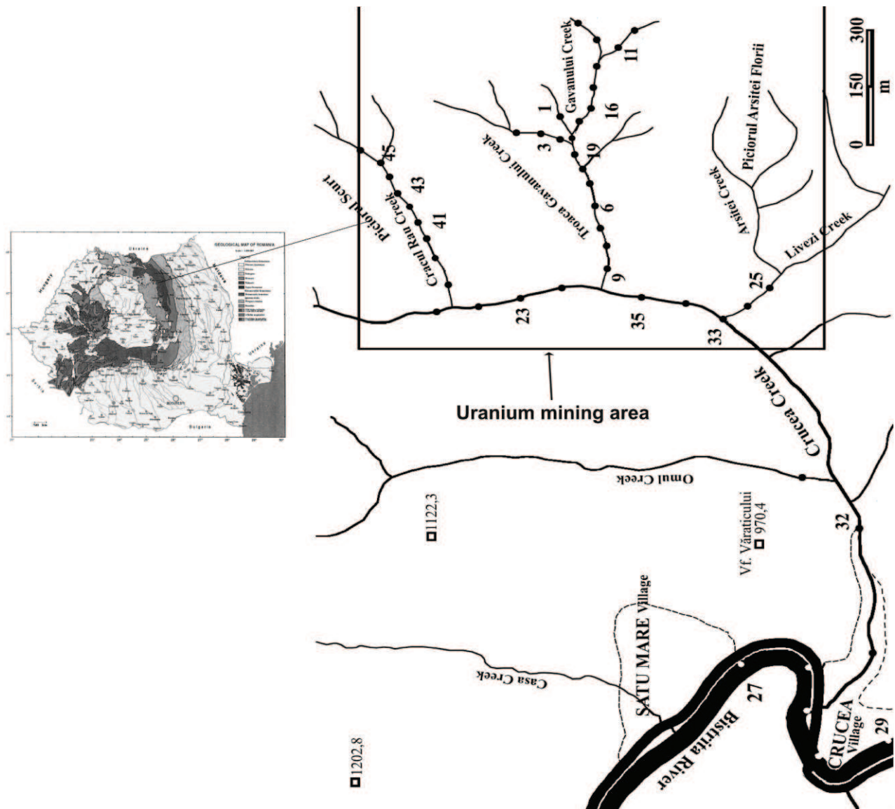
Fig. 1. Topographic map of the investigated area with the distribution of sampling points.
