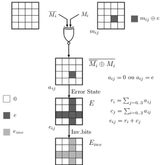
Fig. 7: The Error Detection and Spreading Mechanism
