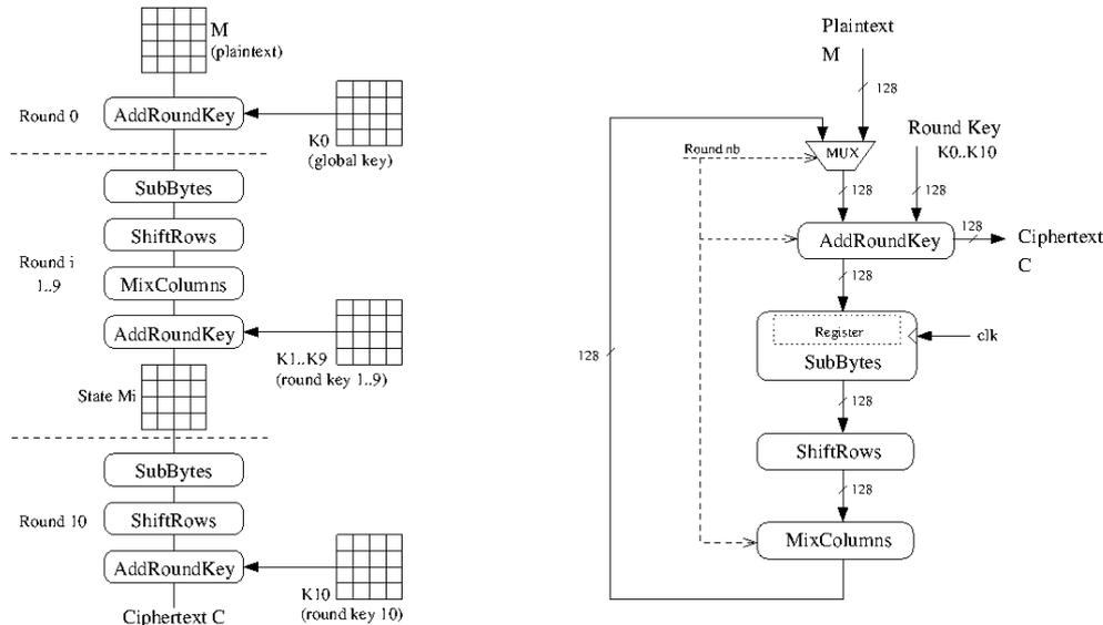
Fig. 5: The AES algorithm and its hardware implementation
