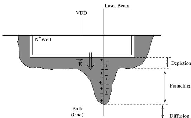
Fig. 1: Laser beam effect onto MOS structure
