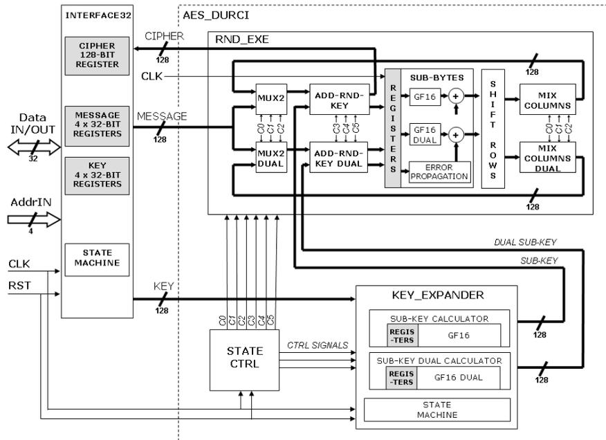
Fig. 6: Overview of the ASIC AES architecture
