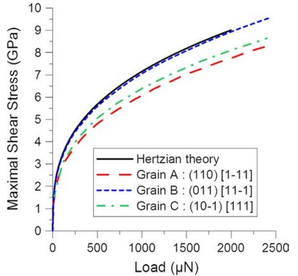
Fig. 7. Resolved shear stresses versus applied load in grains A, B and C and maximal shear stress calculated with the Hertzian contact based isotropic model. The corresponding slip systems of the highest Schmid factor for the three grains are given in the legend.
