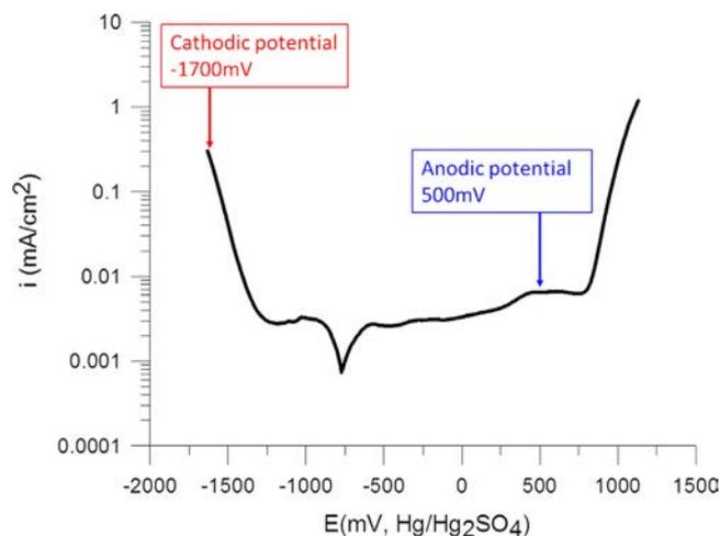
**Fig. 3.** Polarization curve of Fe–15Cr in 0.05 M Na<sub>2</sub>SO<sub>4</sub> with a sweeping rate of 10 mV/s.
