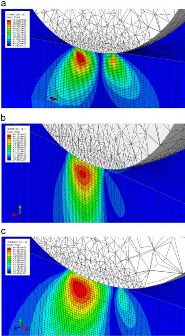
**Fig. 8.** (a) Resolved shear stress distribution in the slip system  $(110)[1-11]$  under the indenter in grain A. Stresses are given in MPa. (b) Resolved shear stress distribution in the slip system  $(011)[11-1]$  under the indenter in grain B. Stresses are given in MPa. (c) Resolved shear stress distribution in the slip system  $(10-1)[111]$  under the indenter in grain C. Stresses are given in MPa.
