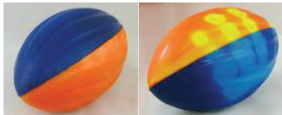
Figure 1 Thermochromic ball: when heated by putting the hand on it, the ball changes colour, LRCHallcrest, source: http://lcrhallcrest.com .
