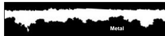
Figure 24. Binary Cr mapping of image presented in Figure 23. Specimen 1594-T112-06 (304L), in site 1B.
