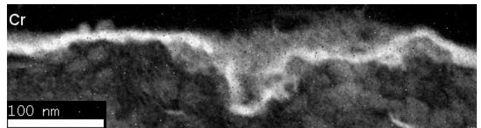
Figure 19 – EFTEM map of Cr-rich inner oxide layer at the surface of specimen 1171H4 (pH 8 – 600h)
