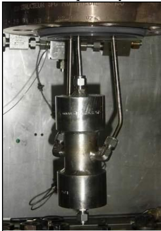
Figure 2 – Capsule for short exposure to primary water. Figure 3 – Evolution of the temperature during testing in capsule.
