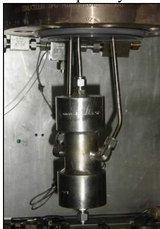
Figure 2 – Capsule for short exposure to primary water.
