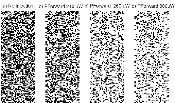
Fig. 4. Fault occurrence rate versus pulse amplitude [4].
