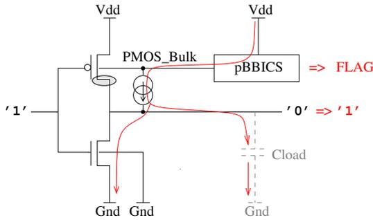
Figure 3: PMOS sensitivity monitoring with a pBBICS.
