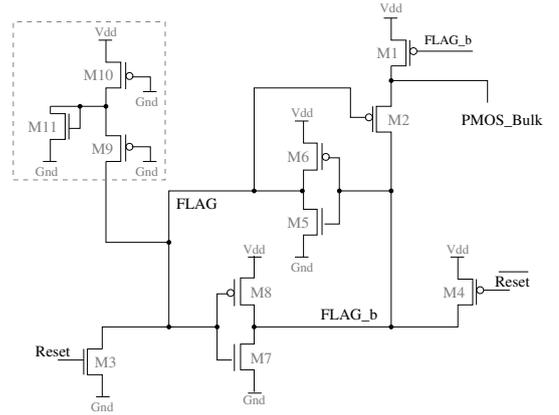
Figure 4: Tbulk BICS architecture for PMOS monitoring [2].
