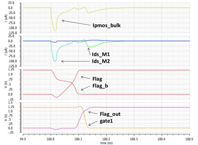
Figure 8: Improved pBBICS waveforms during SEE detection.
