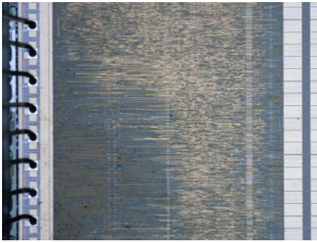
Fig. 6. Decapsulated chip (closeup on SRAM).
