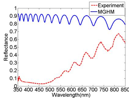
Fig. 2. Experimental specular reflectance of the here studied sample for an incidence angle equal to  $45^\circ$  (dashed red curve) and calculated specular reflectance considering the Maxwell-Garnett homogenization model (MGHM, solid blue curve) for porous alumina film.
