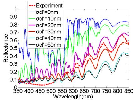
Fig. 4. (All solid curves) Simulated reflectance spectra for a RCWA elementary cell consisting of  $N = 25$  nanopores, with the standard deviation  $\sigma_{cl'}$ , increasing from 0 nm to 50 nm in steps of 10 nm. Each spectrum is calculated for  $P = 30$  random drawings of the elementary cell, for TE and TM polarizations and with a number of Fourier harmonics  $N_{harm} = 4N$  respectively, and finally averaged. The dotted red curve corresponds to the experimental data.
