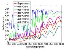
Fig. 4. (All solid curves) Simulated reflectance spectra for a RCWA elementary cell consisting of N=25 nanopores, with the standard deviation  $\sigma_{cl}$ , increasing from 0 nm to 50 nm in steps of 10 nm. Each spectrum is calculated for P=30 random drawings of the elementary cell, for TE and TM polarizations and with a number of Fourier harmonics  $N_{\text{harm}}=4N$  respectively, and finally averaged. The dotted red curve corresponds to the experimental data.
