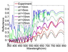
Fig. 5. (All solid curves) Simulated reflectance spectra for a RCWA elementary cell consisting of N=25 nanopores, with the standard deviation  $\sigma_r$ , of the nanopores radius increasing from 0 nm to 25 nm in steps of 5 nm. Each spectrum is calculated for P=30 random drawings of the elementary cell, for TE and TM polarizations and with a number of Fourier harmonics  $N_{\rm harm}=4N$  respectively, and finally averaged. The dotted red curve corresponds to the experimental data.
