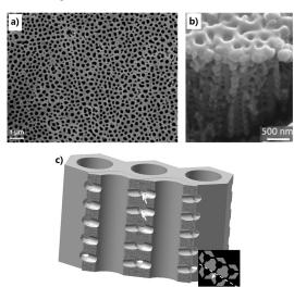
Fig. 1. (a) Top view of SEM measurement results of our fabricated partially ordered nanoporous alumina film on aluminum substrate, (b) side view of a fractured part of the same sample and (c) 3D-scheme of the porous morphology.
