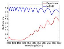
Fig. 2. Experimental specular reflectance of the here studied sample for an incidence angle equal to 45° (dashed red curve) and calculated specular reflectance considering the Maxwell-Garnett homogenization model (MGHM, solid blue curve) for porous alumina film.
