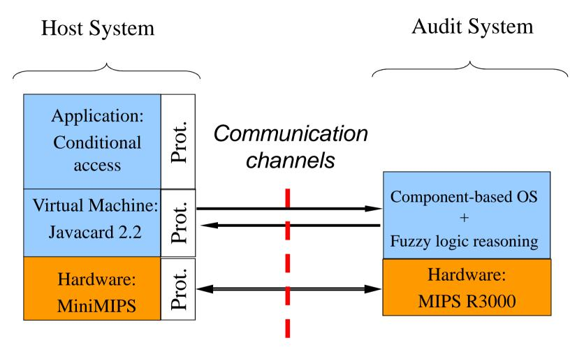
Transfers of sensor values and of parameters of protection BUT NO TRANSFERT OF SENSITIVE DATA!!
