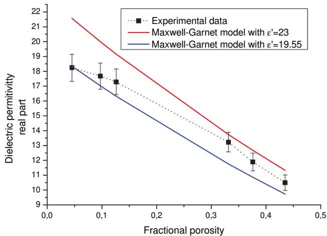
**Fig. 9.** Variation of the relative dielectric properties (real part)  $\epsilon'$  versus the fractional porosity and the Maxwell-Garnet models.
