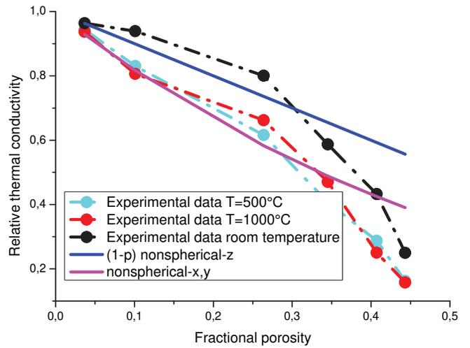
**Fig. 8.** Variation of the relative thermal conductivity  $\lambda/\lambda_0$  versus the fractional porosity at room temperature (black) 500 °C (cyan) and 1000 °C (red) compared with two models. (For interpretation of the references to color in this figure legend, the reader is referred to the web version of this article.)
