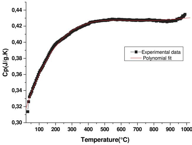
Fig. 3. Heat capacity for the CeO<sub>2</sub> powder in argon.
