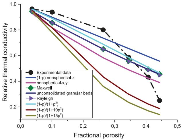
**Fig. 7.** Variation of the relative thermal conductivity  $\lambda/\lambda_0$  versus the fractional porosity at room temperature from our experiments (black) compared with different models from [15–21].
