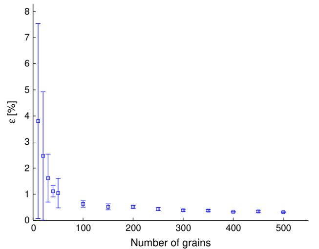
**Fig. 3.** Validity criterion of the flux superposition hypothesis.
