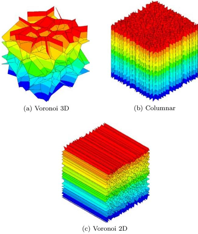
**Fig. 2.** Grain shapes used to perform simulations. Diffusion direction is vertical, highlighted by the color gradient. (For interpretation of the references to colour in this figure legend, the reader is referred to the web version of this article.)
