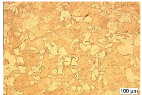
Fig. 13. Grain structure of the commercially pure copper.
