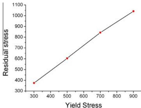
Fig. 15. Evolution of residual stress versus yield stress.
