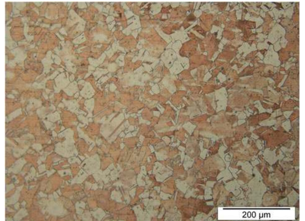
FIG. 5. Grain size of commercially pure copper.
