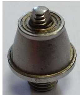
Figure 2: Triflat FSW tool used for the welding trials.
