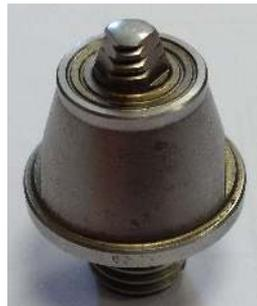
Figure 2: Triflat FSW tool used for the welding trials.
