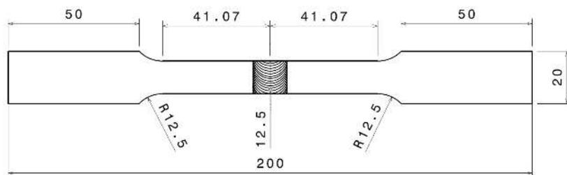
Figure 4: Tensile samples geometry (thanks to ASTM-E8 standard).
