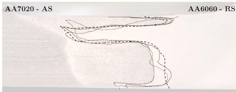
Figure 8: Interfaces repeatability (4 times) for BW7 condition.
