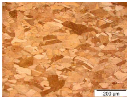
Figure 1: Optical micrograph showing the initial microstructure of the copper bar.
