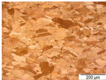
Figure 1: Optical micrograph showing the initial microstructure of the copper bar.
