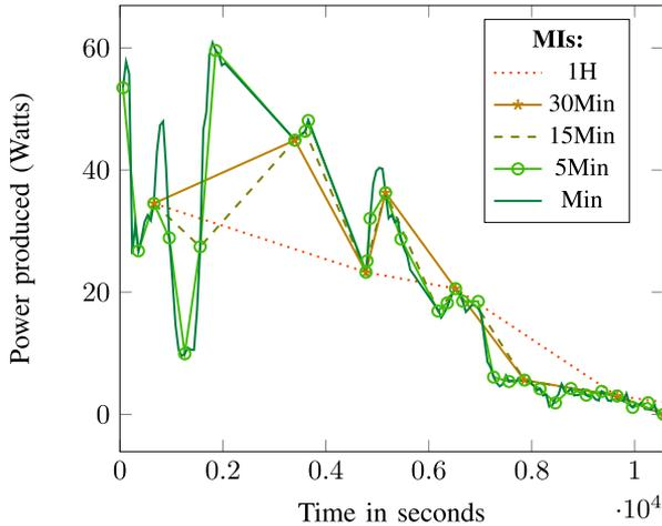
Fig. 5. PV production measurement differences with various MIs.
