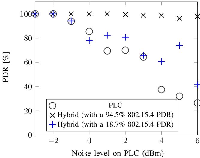
Fig. 9. PDR depending on noise level over PLC line.
