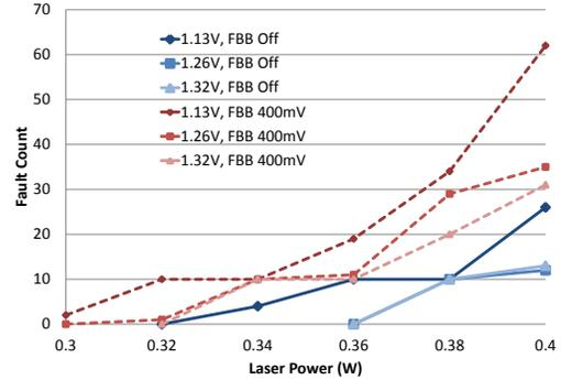
Fig. 3: Faults for different laser power values
