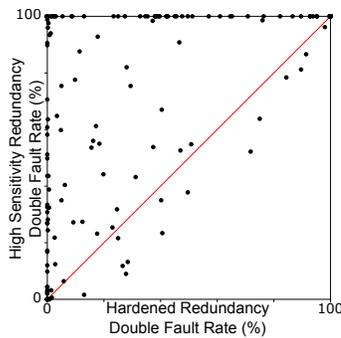
Fig. 6: Double fault success rates (hardened vs. high-sensitivity)
