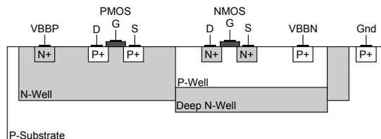
Fig. 1: Cross-sectional view of CMOS Triple-Well process
