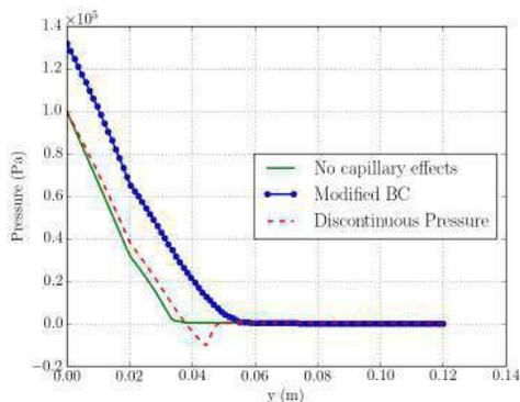
Figure 15: Comparison of the pressure fields with the *Modified BC - Discontinuous Pressure* methods and without capillary effects at  $t=3000s$  along a vertical line  $\{0.01; y; 0.2\}$  plotted in Fig. 14b.
