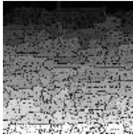
Figure 23.4: Even if the gradient is performed on the filtered image, there is still a high over-segmentation.
