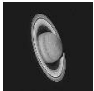
(h) Landweber iterative deconvolution with 200 iterations and Jansson parameter at 1.
