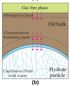
Figure 1. (a) Gas-(water-in-oil) slug flow gives rise to hydrate particles with size similar to the water droplets. (b) Gas mass transfer process up to the capillary walls where crystallization occurs.
