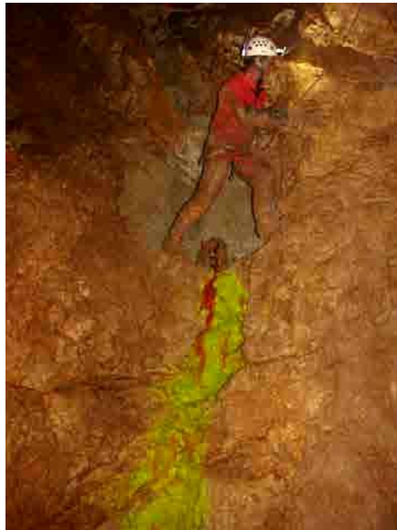
Photo 1: Injection de 10kg de fluorescéine dans la grotte Flandin le 29mars 2014 (photo: GASOIL) Injection of 10 kg of fluoresceine into Flandin Cave on March 29, 2014 (photo: GASOIL)
