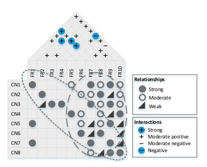
Figure 7. House of Quality—FRs' identification based on CNs.
