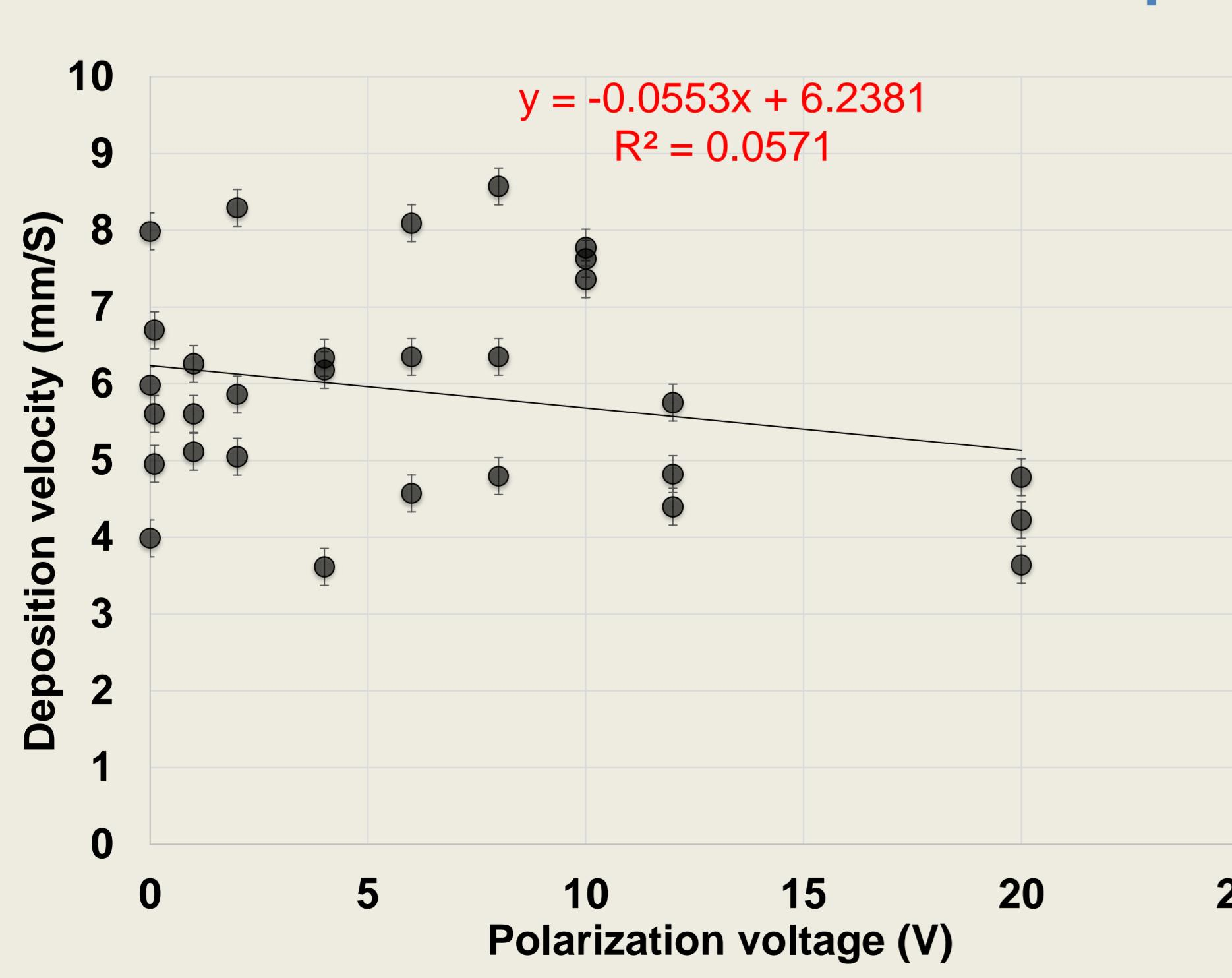
→ Same deposition velocity under low polarization voltage (0 to 20 V)
