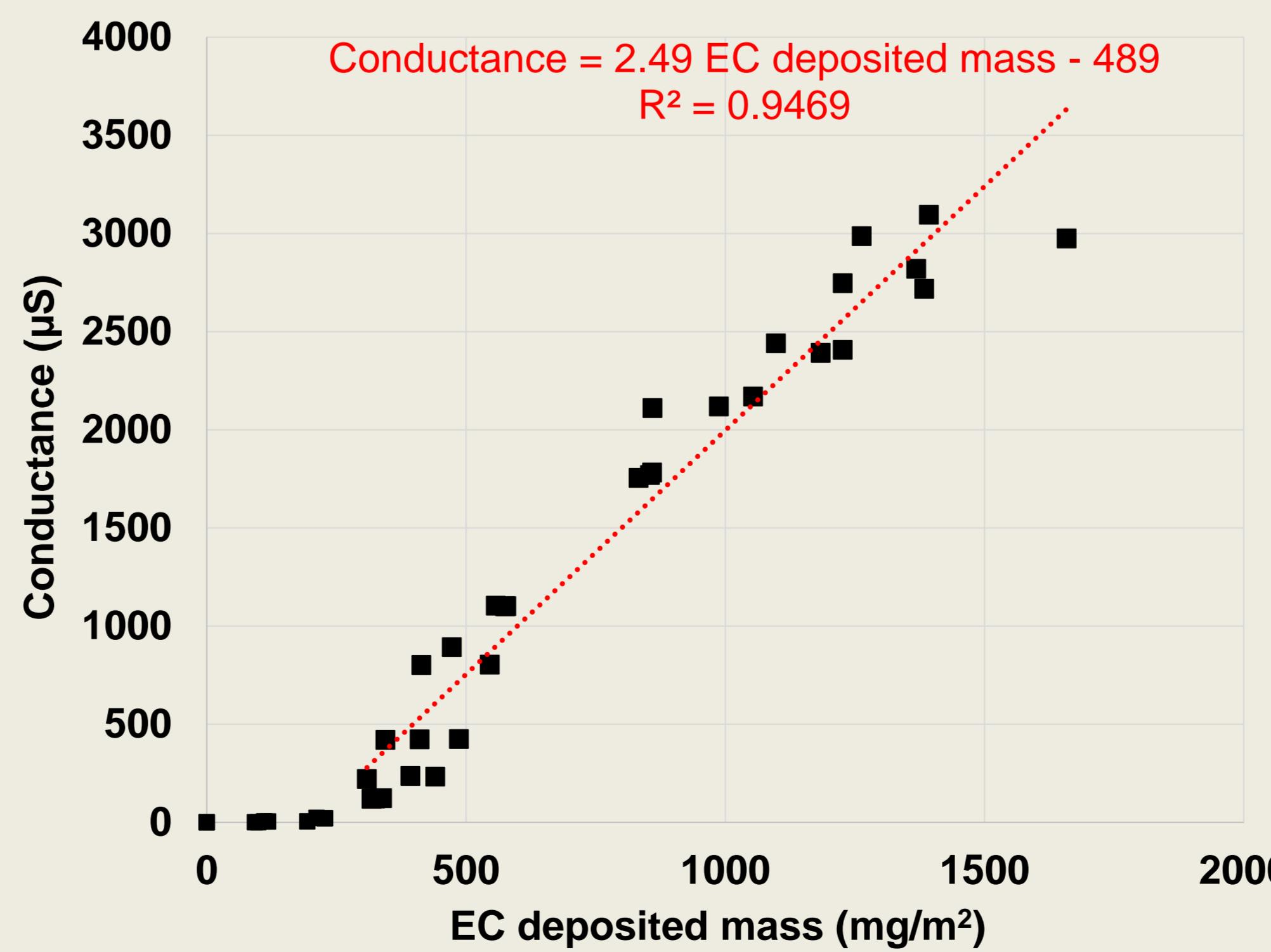
→ Mass to conductance correlation at a polarization voltage of 10 V
