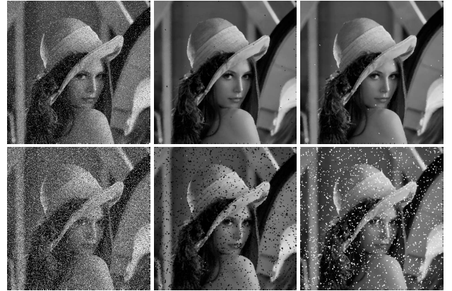
Fig. 1: From left to right. Up to down. first column: images with impulsive noise of 10% and 30%; second column: morphological filter \gamma_B \phi_B \gamma_B ; third column: morphological filter \phi_B \gamma_B \phi_B . B is the diamond-shaped structuring element.
