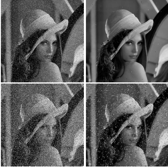
Fig. 2: . From left to right. Up to down. First column: images with impulsive noise of 10% and 30%; second column: morphological center C(f) where B is the diamond-shaped structuring element.
