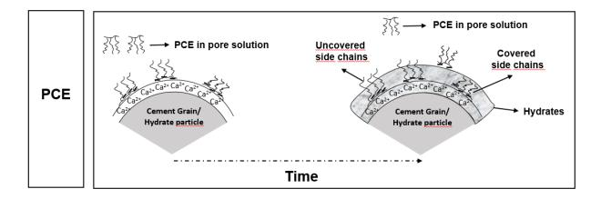
Fig. 14 Acting mechanism of PCE
