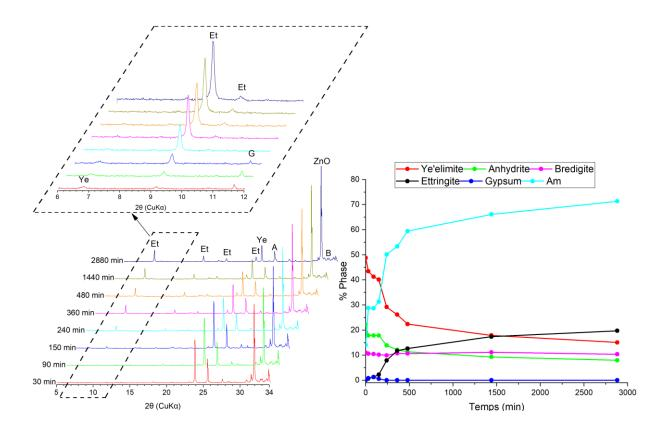
Fig. 4 diffraction patterns of 0.2AC after several times of hydration (left) ; phase evolution during the hydration of 0.2AC (right). Et: ettringite, G: gypsum, Ye: ye'elimite, A: anhydrite,
