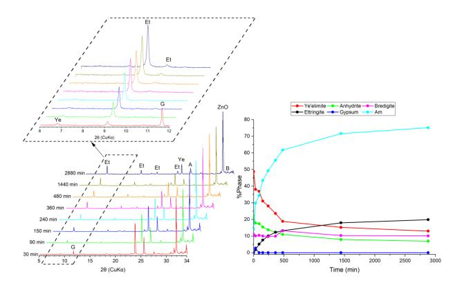
Fig. 3 diffraction patterns of CSA after several times of hydration (left); phase evolution during the hydration of CSA (right). Et: ettringite, G: gypsum, Ye: ye'elimite, A: anhydrite,
