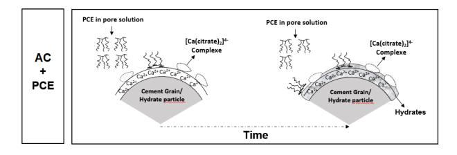
Fig. 15 Acting mechanism of AC+PCE
