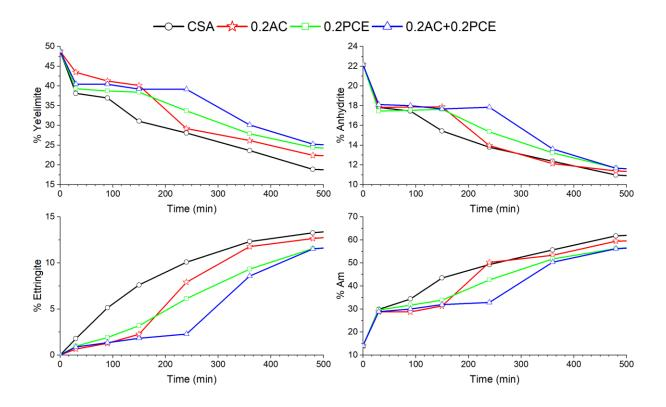
Fig. 7 Evolution of the amount of anhydrous and hydrated phases of CSA, influenced by AC,PCE and their combination. Results were derived from the Rietveld calculations. The dosage of admixtures was fixed at 0.2 wt%.
