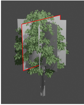
Figure 1: A tree and its equivalent in the model with 4 vertical rectangles (a single vertical rectangle is highlighted with red borders).
