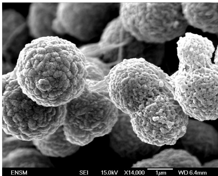
Fig. 2. Multi-scale ZnS agglomerate
