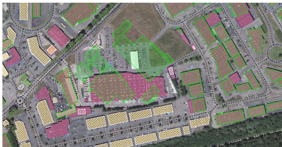
Figure 4. Temporal snapshots overlapped with an orthophotograph from 2020. Buildings captured at different dates are shown with green and white strokes for 2004 and rose and beige solid color for 2019. Unless the terrain changes, they are perfectly identical from one database version to the next.
