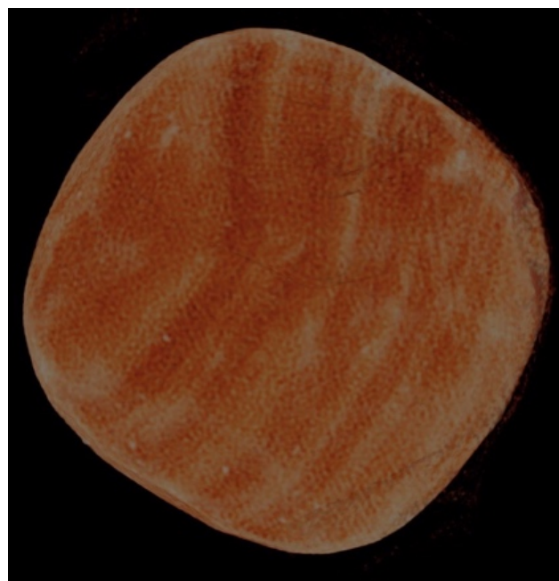
Figure 8. Computed tomography (CT) scan reconstruction of the wooden model. Homogeneity. Largest diameter 65 mm.
