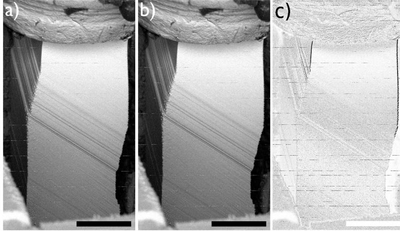
Supplementary Figure 9: **Locating spatial distribution of a strain burst.** a, b, Backscattered electron images of the micropillar before and after the stress drop analysed in Figs. 1c-e. The scale bar represents 20  $\mu\text{m}$ . c, The difference of panels a) and b). The dark edges at the upper part of the pillar are due to plastic slip that occurred on the slip band highlighted in red in Fig. 1b.
