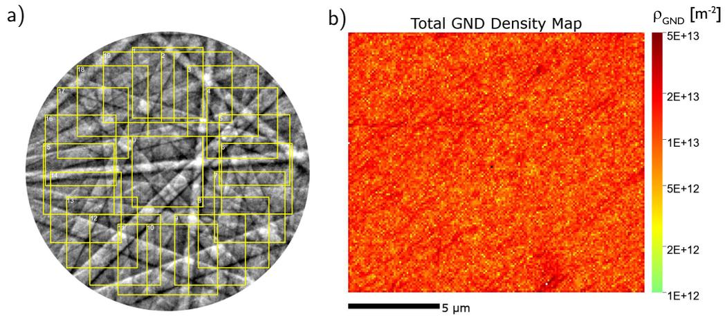
Supplementary Figure 5: **a**, A typical Kikuchi pattern collected from the sample used for the HR-EBSD evaluation. 20 regions of interest are marked with yellow squares. **b**, The resulting GND density map. Black point (in the middle) marks the reference pixel.
