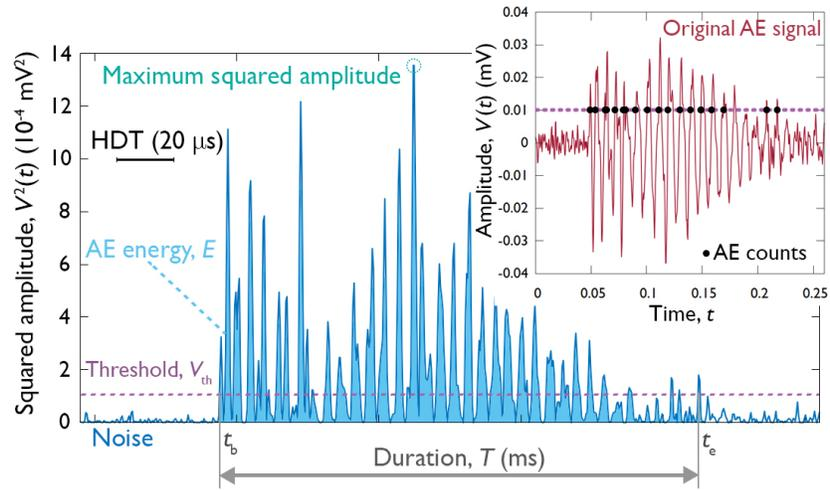
Supplementary Figure 11: **Parameters of a typical AE event.** Squared amplitude  $V^2(t)$  of the AE signal as a function of time, showing the definitions of the AE parameters. The energy is the area of the region shaded in light blue. The inset presents the original waveform.
