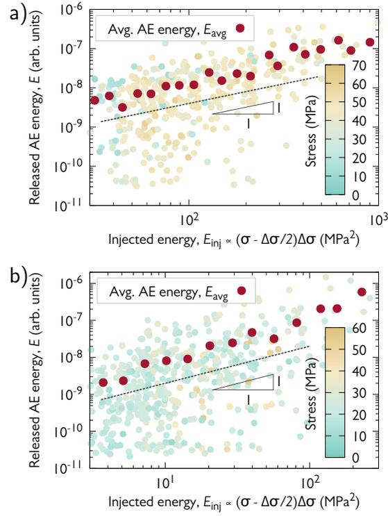
Supplementary Figure 3: **Correlation between stress drops and released AE energy.** **a**, Equivalent figure to that of Fig. 2c for  $d = 8 \mu\text{m}$  micropillars. **b**, Equivalent figure to that of Fig. 2c for  $d = 16 \mu\text{m}$  micropillars.
