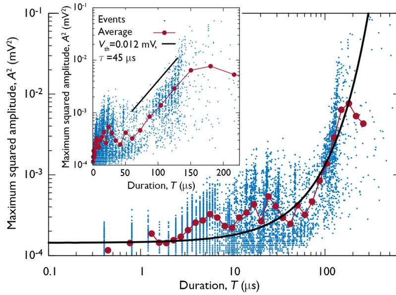
Supplementary Figure 12: **Analysis of AE signal attenuation.** Scatter plot of the maximum squared amplitude of individual AE events and their duration. The red data points represent the average relationship obtained by logarithmic binning with respect to the signal duration. Black solid line corresponds to the fit according to Eq. (8).
