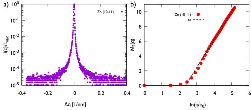
Supplementary Figure 6: **X-ray diffraction measurements on the original bulk Zn sample.** **a**, The measured X-ray line profile of the  $(10\bar{1}1)$  reflection of the Zn single crystal. **b**, Second restricted moment  $M_2$  as a function of  $\ln q/q_0$ , with  $q_0 = 1.0$  1/nm. Dislocation density can be obtained from the linear fit from Eq. (1).
