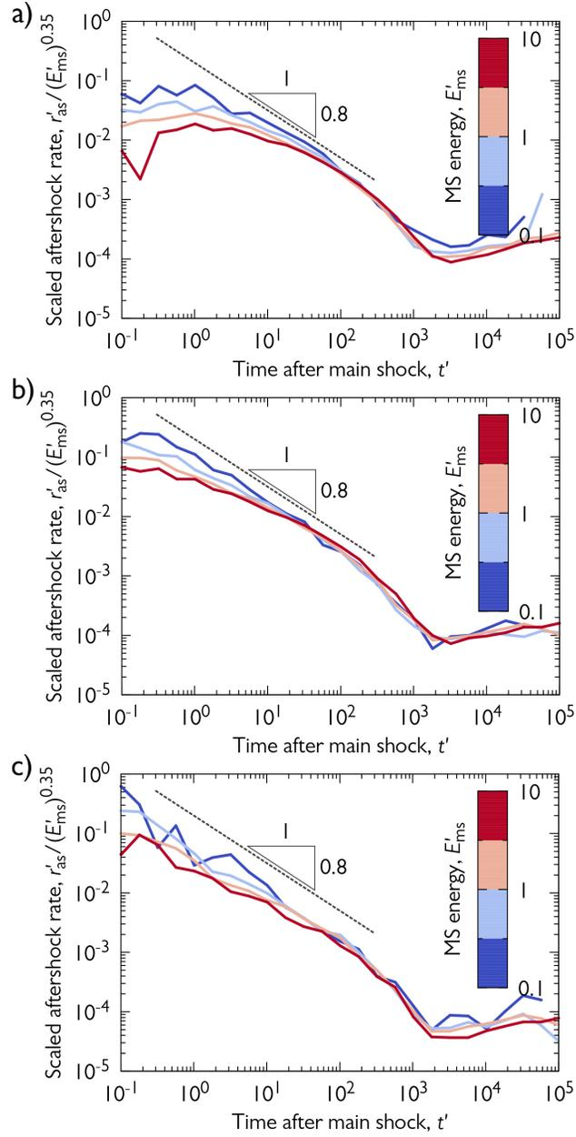
Supplementary Figure 16: **Effect of thresholding on the emulated scaled aftershock rates in DDD simulations.** Aftershock rates  $r'_{as}$  after main shocks with different energies  $E'_{ms}$  scaled with  $(E'_{ms})^{0.35}$ . The panels correspond to rates observed at different thresholds  $r'_{th,AE}$  used for the emulation of AE events: **a**,  $r'_{th,AE} = 0.1$ . **b**,  $r'_{th,AE} = 1$ . **c**,  $r'_{th,AE} = 10$ .
