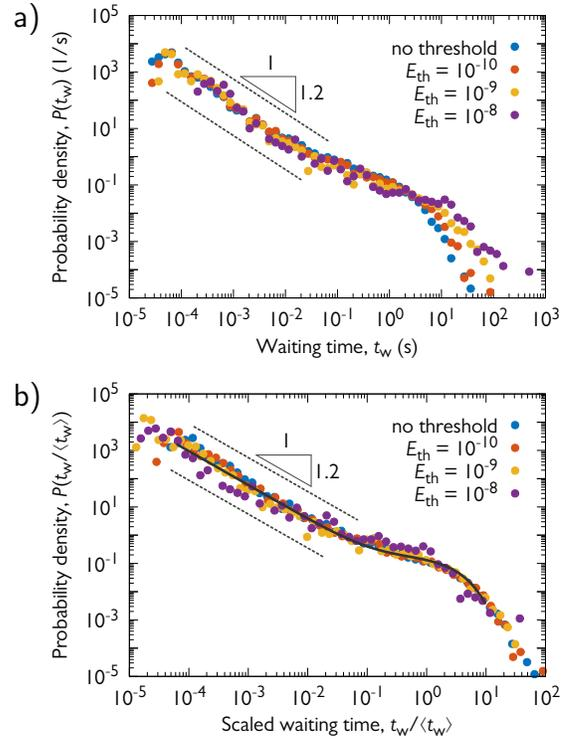
Supplementary Figure 13: **Effect of thresholding on waiting time distributions of  $d = 32 \mu\text{m}$  micropillars.** **a**, Waiting time distributions for AE events with energies larger than  $E_{th}$ . **b**, Distributions of panel a) re-scaled with the average waiting time of the events. The master curve fitting the collapsed curves is identical to that of Fig. 3f.
