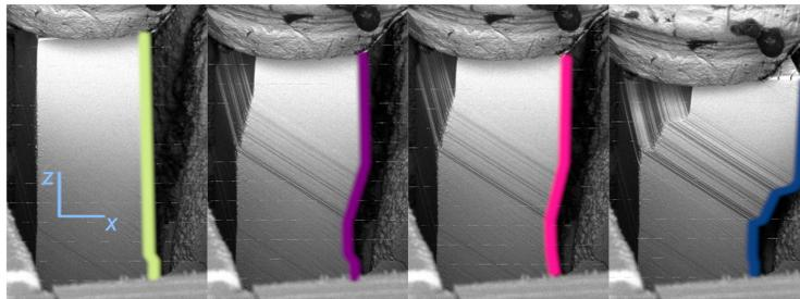
Supplementary Figure 8: **Time development of the right edge of the micropillar.** Distance from the reference line with the corresponding height as a function of time indicated by the colour for the micropillar shown in Fig. 1b. The purple and pink lines indicate the pillar shape before and after the stress drop investigated in Figs. 1c-e, respectively. The light gray horizontal line highlights the place where slip occurred.
