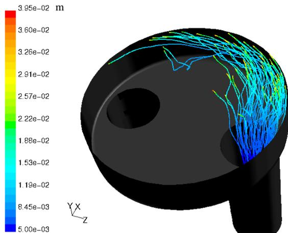
The net argon mass flux going in the ladle, even if it is a small fraction of the total injected mass flux, should also be precisely determined, because it could be an efficient way of improving inclusion elimination. This could be evaluated using a critical Weber number, but having good prediction for  $\epsilon$  is necessary (17).
