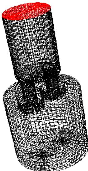
For bubble injection, the diameter is 5 mm and approximately 100 injection points are homogeneously distributed in the section of one snorkel. Each free surface (ladle and RH) corresponds to non-slip condition, with "escape through the boundary" for the bubbles (see Figure 3 for the mesh).
