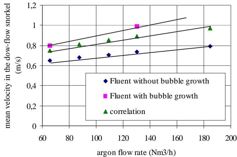
Figure 5 : Comparison of Fluent's results with standard correlation.
