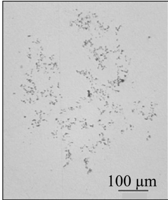
Figure 1 : Typical shape of alumina cluster
