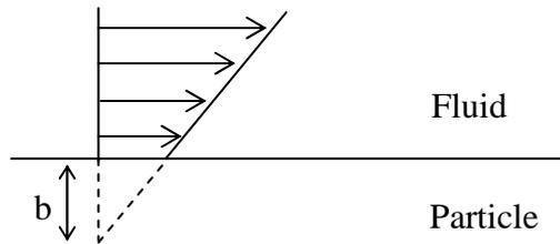
Figure 2 : fluid behaviour for hydrophobic surface
