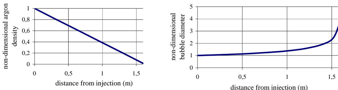
Figure 4 : Dependence of bubble properties on vertical position.
